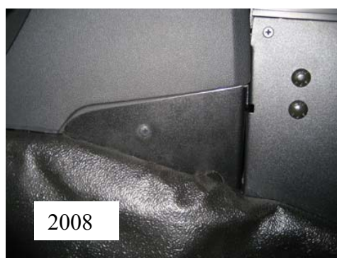
Attach side trim panels using #10 x 1/2" machine screw & washer (Phillips screwdriver) (Item 3)
